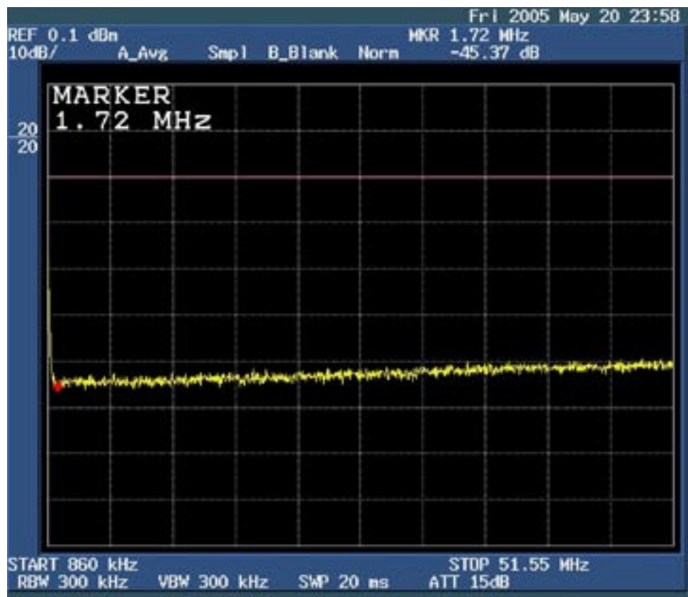
Figure 2. Return Loss of 75\Omega Test Load
