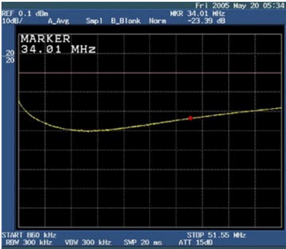
Figure 6. Return Loss of the DS3150DK with Modified Termination Network at 34.01MHz
